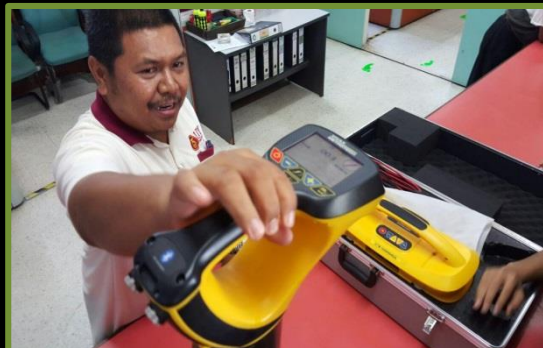
Demonstrasi Peralatan Pipe & Cable Locator (PCL)
